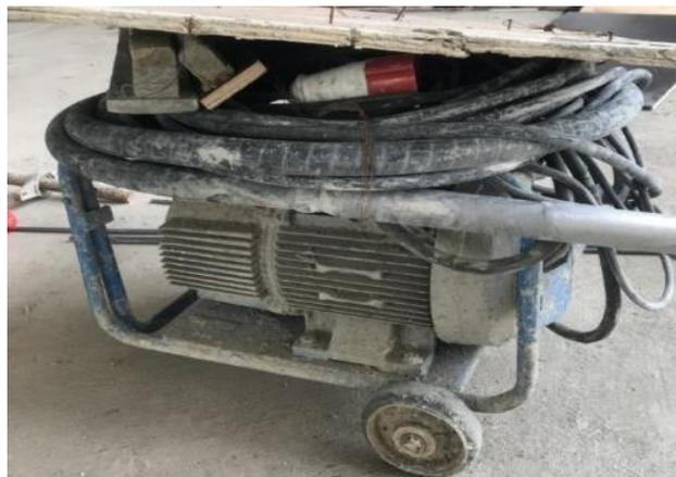
Gambar 4.23. *Concrete vibrator*
