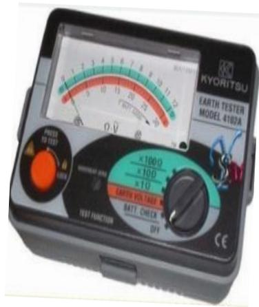
**Gambar 3.4 Earth tester analog**
