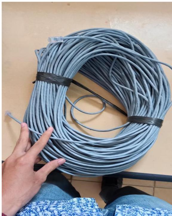
**Gambar 4. Kabel LAN Twisted pair tipe UT**
