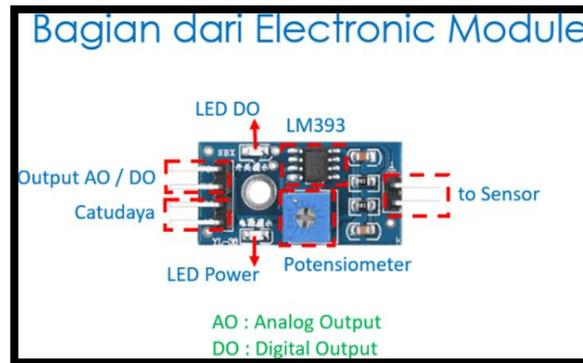
Gambar 3.3. Bagian *electronic* modul
