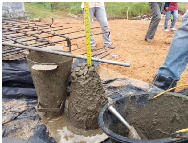
Gambar 4.1. Slump Test Beton
