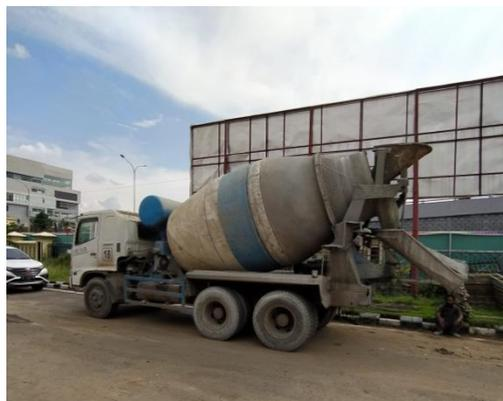
**Gambar 3.12** *Ready Mixed Concrete Truck*
