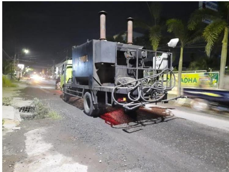
*Gambar 3.8 Asphalt Sprayer*
