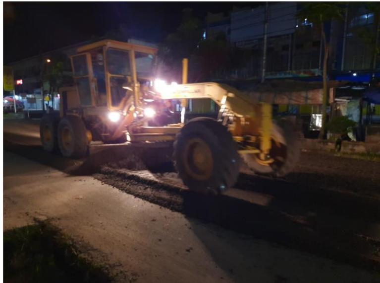
*Gambar 3.4 motor grader*
