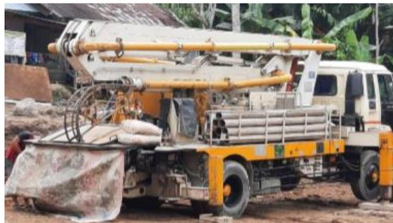
Gambar 4.4 *Concrete Pump Truck*
