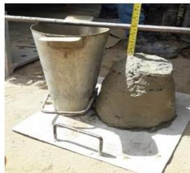
Gambar 5.1 Pengujian *Slump Cone Test*
