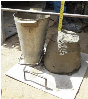
Gambar 4.26 Pengujian *Slump Cone Test*
