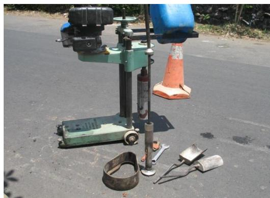
Gambar 4.3 Alat Core Drill
