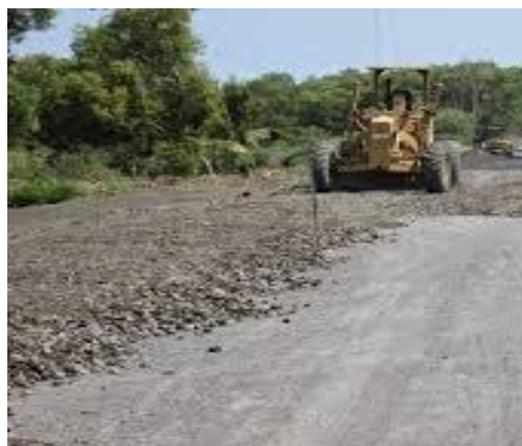
Gambar 3.1 Motor grader
