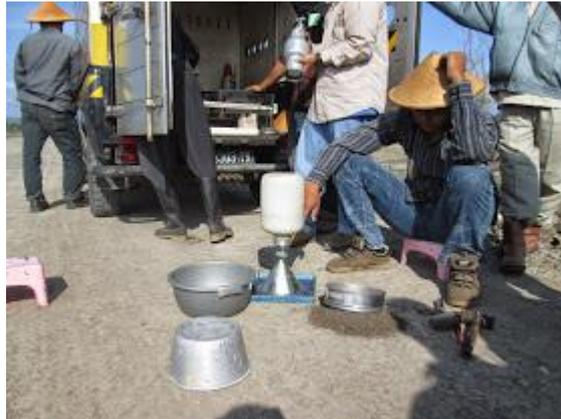
Gambar 4.2 Uji Sand Cone
