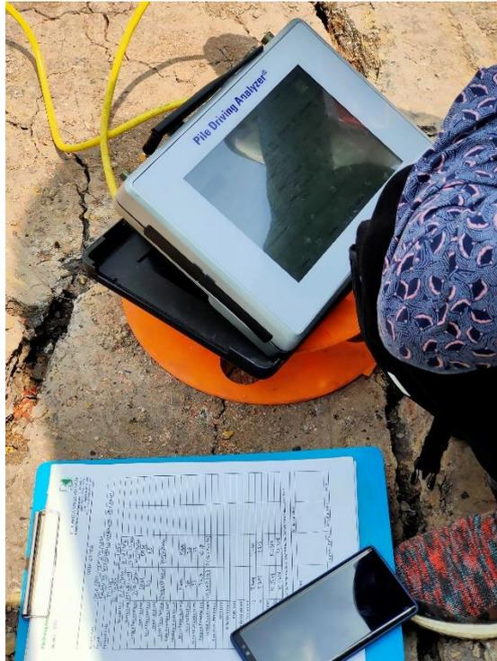
Gambar 4.15 Alat Pile Driving Analyzer (PDA) Test
