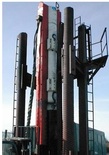
Gambar 3.6 Double-Acting Hammer
