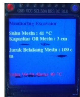
Figure 7 Lcd display when temperature above 40oC
