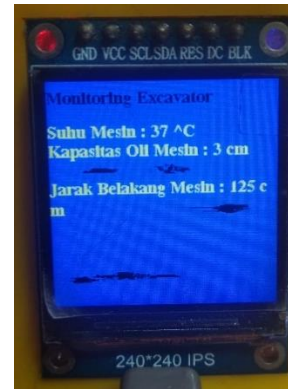
Figure 5 Lcd display when normal
