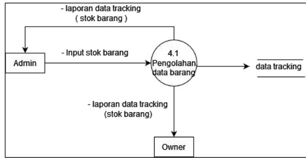
Gambar 8. Data Flow Diagram DFD Level 1 Proses Pengolahan Data Barang
