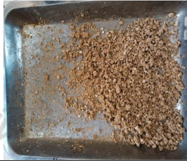
Gambar 13. Persiapan Sampel 1-D Free Swell Test
