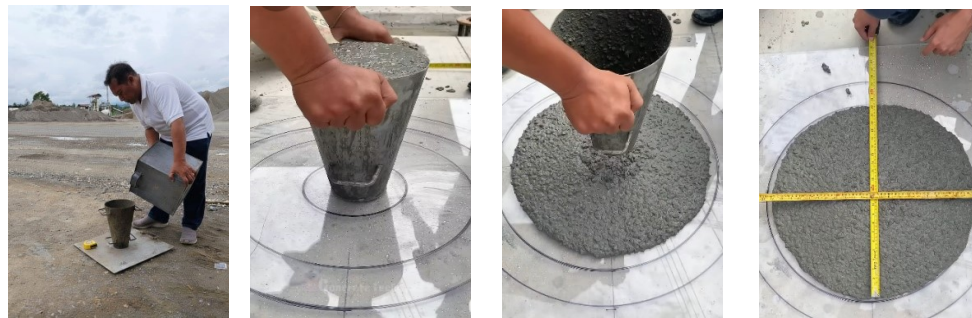
Gambar 4. 3 kegiatan Flow Test
